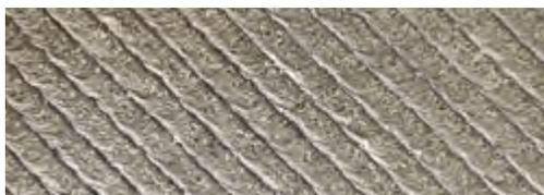
The 45 degree orientation of the welding bead to the conveying direction induces only small wear. Welding toes as well as hardening cracks are directed at a 45 degree angle to the conveyor stream, protecting the component against wear.
