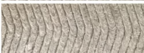
Wearout during transportation of highly abrasive media is often evident at welding transitions. If high speed transportation of highly abrasive or very fine particles is needed, the welding in sine wave form should be preferred because it shows great advantages in reduced wear of the component.
