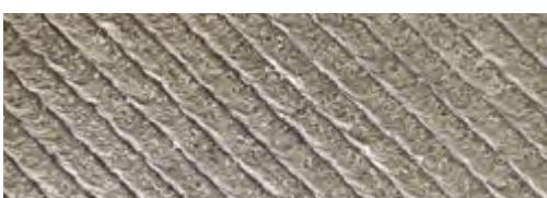
The 45 degree orientation of the welding bead to the conveying direction induces only small wear. Welding toes as well as hardening cracks are directed at a 45 degree angle to the conveyor stream, protecting the component against wear.
