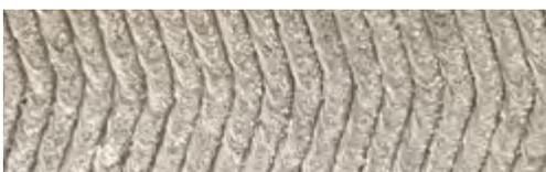
Wearout during transportation of highly abrasive media is often evident at welding transitions. If high speed transportation of highly abrasive or very fine particles is needed, the welding in sine wave form should be preferred because it shows great advantages in reduced wear of the component.
