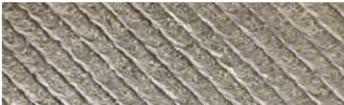
The 45 degree orientation of the welding bead to the conveying direction induces only small wear. Welding toes as well as hardening cracks are directed at a 45 degree angle to the conveyor stream, protecting the component against wear.
