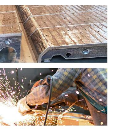
By using flux-cored electrodes, our manufacturing process reliably guarantees the highest coating quality. This process is characterised by the even distribution of hard carbides along the entire weld metal area and extremely low fusion with the actual base material.
